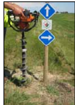
A gas-powered, post-hole auger was rented to save an extra tractor rental.
